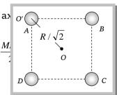
$I_O = I_{O'} + M \left(\frac{R}{\sqrt{2}}\right)^2 = \frac{2}{5}Mr^2 + \frac{MR^2}{2}$  [by the theorem of parallel ax Moment of inertia of system (i.e. four sphere) =  $4I_O = 4\left[\frac{2}{5}Mr^2 + \frac{M}{2}\right]$
