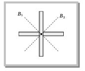
Solution: (b) Moment of inertia of system about an axes which is perpendicular to plane of rods and passing through the common centre of rods  $I_z = \frac{Ml^2}{12} + \frac{Ml^2}{12} = \frac{Ml^2}{6}$
